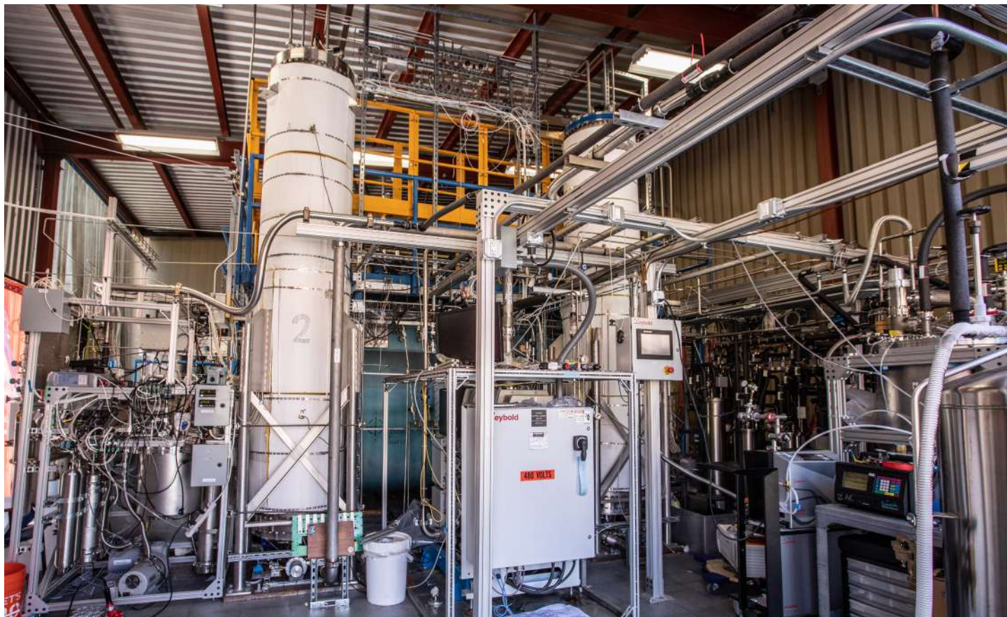
Xenon purification system for the LZ experiment at SLAC. Photo: Jacqueline Orrell, SLAC
