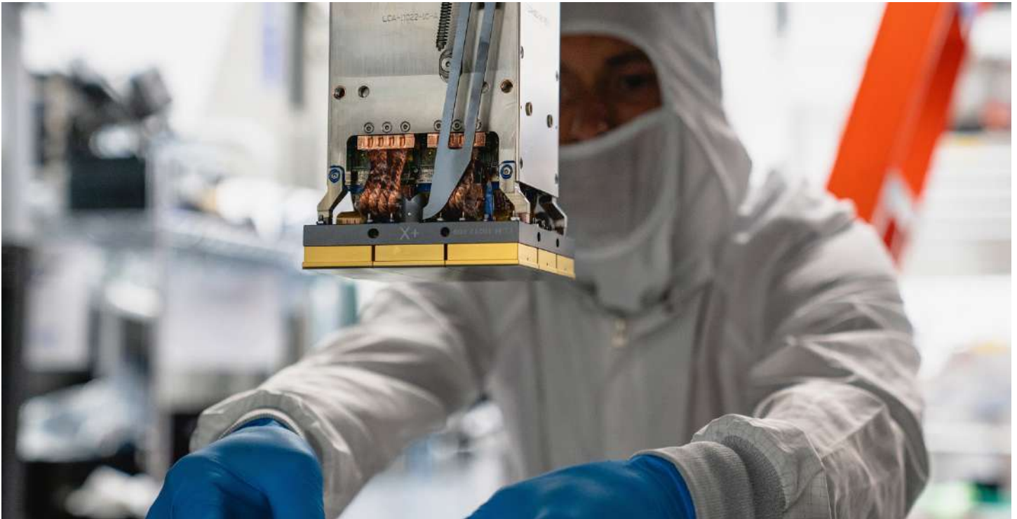
An engineer checking one of the science rafts comprising LSST Camera's focal plane. Photo: Travis Lange, SLAC
