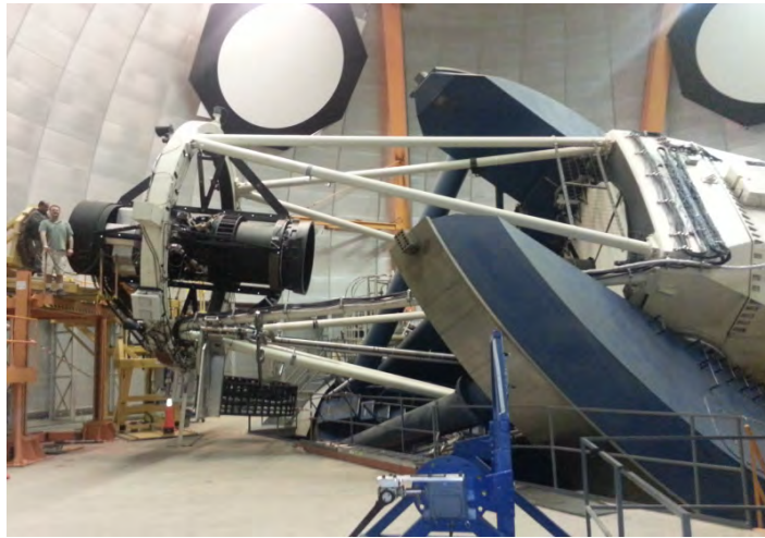
DECam at the Blanco telescope—I am one of the small humans on the left, DECam is the large black cylinder next to us, and what's on the right is not a crashed cousin of the Millennium Falcon but the actual telescope mechanism that holds the mirrors and focuses the light that ends up being imaged in DECam.
